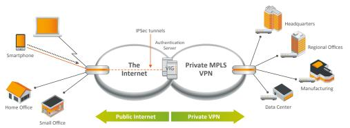
It can be quite cost-effective to use IPsec VPN services in highly dispersed organizations with lots of small locations, such as retail chain stores, restaurants and small bank branches. Regardless of the physical wired or wireless connection type, IPsec VPNs can ultimately terminate directly at the corporate data center or at the enterprise's MPLS VPN point of presence.
